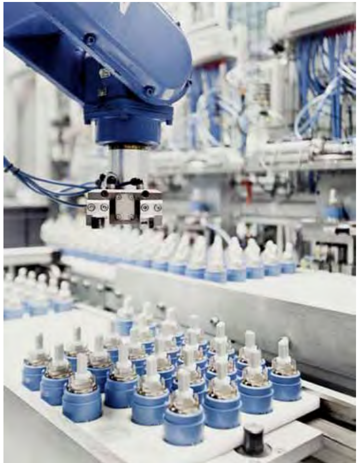
Fully automated functional testing of ceramic inserts.
